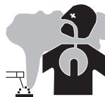
The fumes, gases and dust produced during welding are hazardous. It is mandatory to ensure adequate ventilation and/or extraction to keep fumes and gases away from the work area. An air fed helmet is recommended in cases of insufficient air supply in the workplace. Check that the air intake is in compliance with safety standards.
