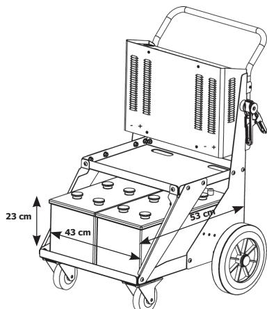
Before any use, instal both « internal batteries » (not provided) : 12V lead batteries with liquid or gel electrolyte of a maximum capacity of 120 to 170 Ah each. Their dimensions must not exceed 45x 53x23 cm, and 100 kg for the total weight.
