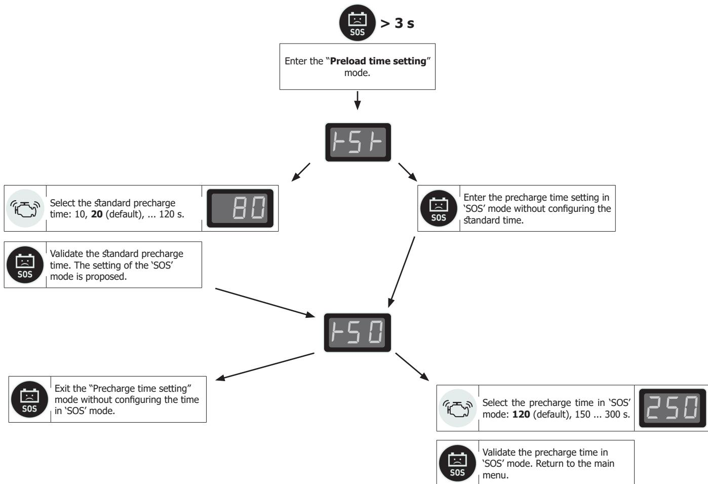
**In SOS mode, there are no more protections (on the 12 V / 24 V voltage, in case of polarity reversal...).**
