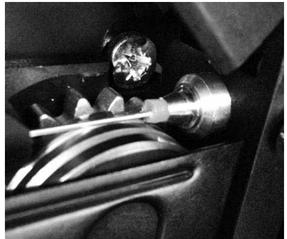
When using a blue or red torch liner (aluminium welding), it is recommended to use accessory 91151 (see picture). This stainless steel guide tube improves the torch liner positioning and facilitates wire feeding.
