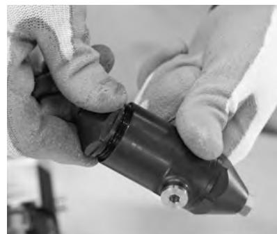
**Tightening torque: 15 N.m**
