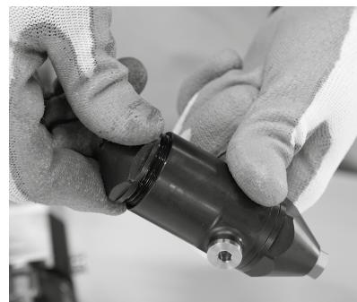
**Tightening torque: 15 N.m**
