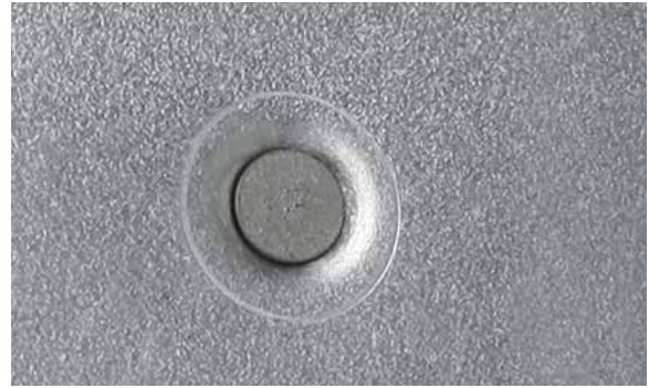
RESULT OF THE INSTALLATION OF SELF-PIERCING RIVET
