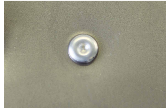
RESULT OF THE INSTALLATION OF A FLOW-FORM RIVET
